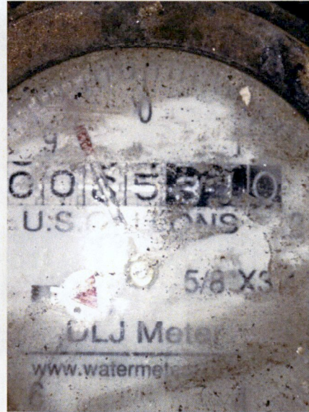
Figure 3. Two water meters purchased and installed on March 20 th , 2014 to measure pen wash down water additions to manure volume. Meters readings were 96,609.6 and 65,319.3 gallons for meter 1 and 2 on September 10 th , 2014.
