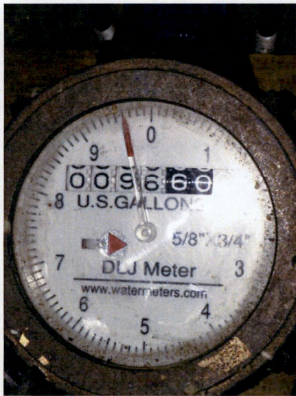
Figure 3. Two water meters purchased and installed on March 20 th , 2014 to measure pen wash down water additions to manure volume. Meters readings were 96,609.6 and 65,319.3 gallons for meter 1 and 2 on September 10 th , 2014.
